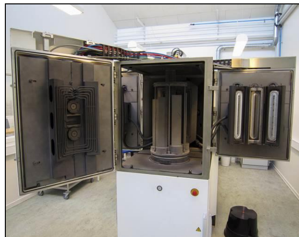
Figure 2 The open PVD vacuum chamber.
