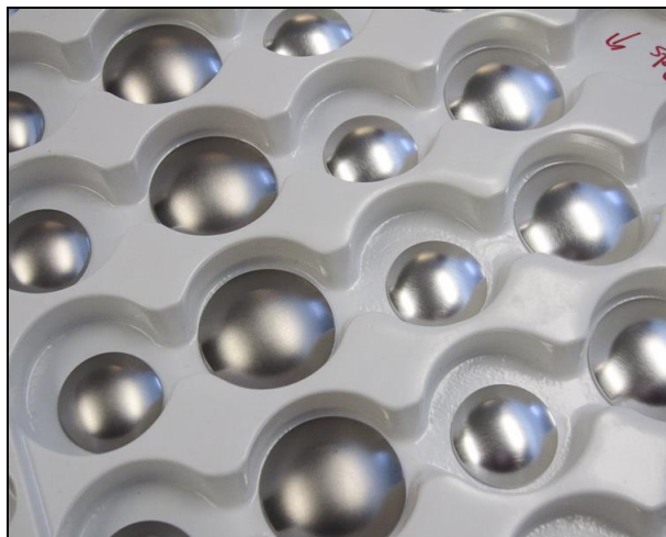
Figure 10 Raw domes (right) and Cr/CrN coated domes.
