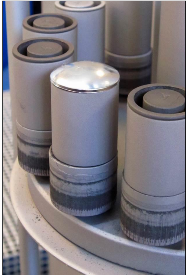
Figure 4 Mounting of raw domes on the carrousel.
