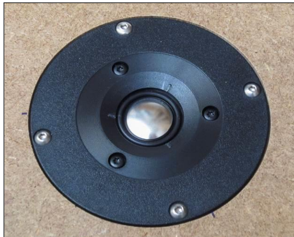
Figure 11 A healthy 19 mm tweeter mounted for test.
